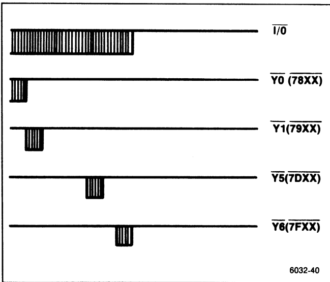
Figure 6-31. Chip selects Y0, Y1, Y5, and Y7 in relation to \overline{T/O} .
